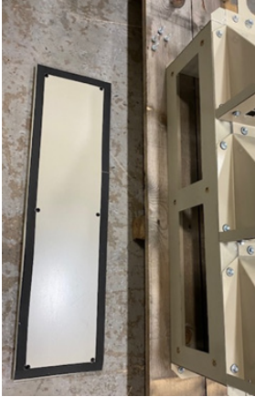
Figure 96: Side flange to be secured once side panel is removed
